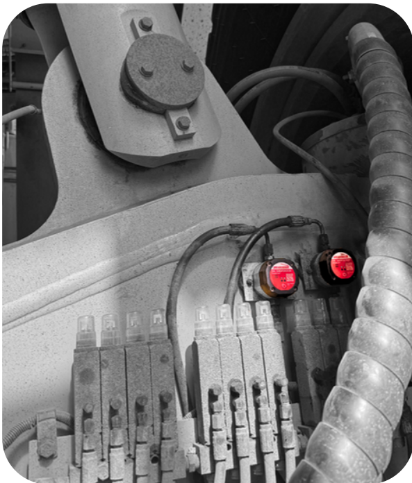
Endpoint LF monitoring kingpins – mounted on magnetic brackets
