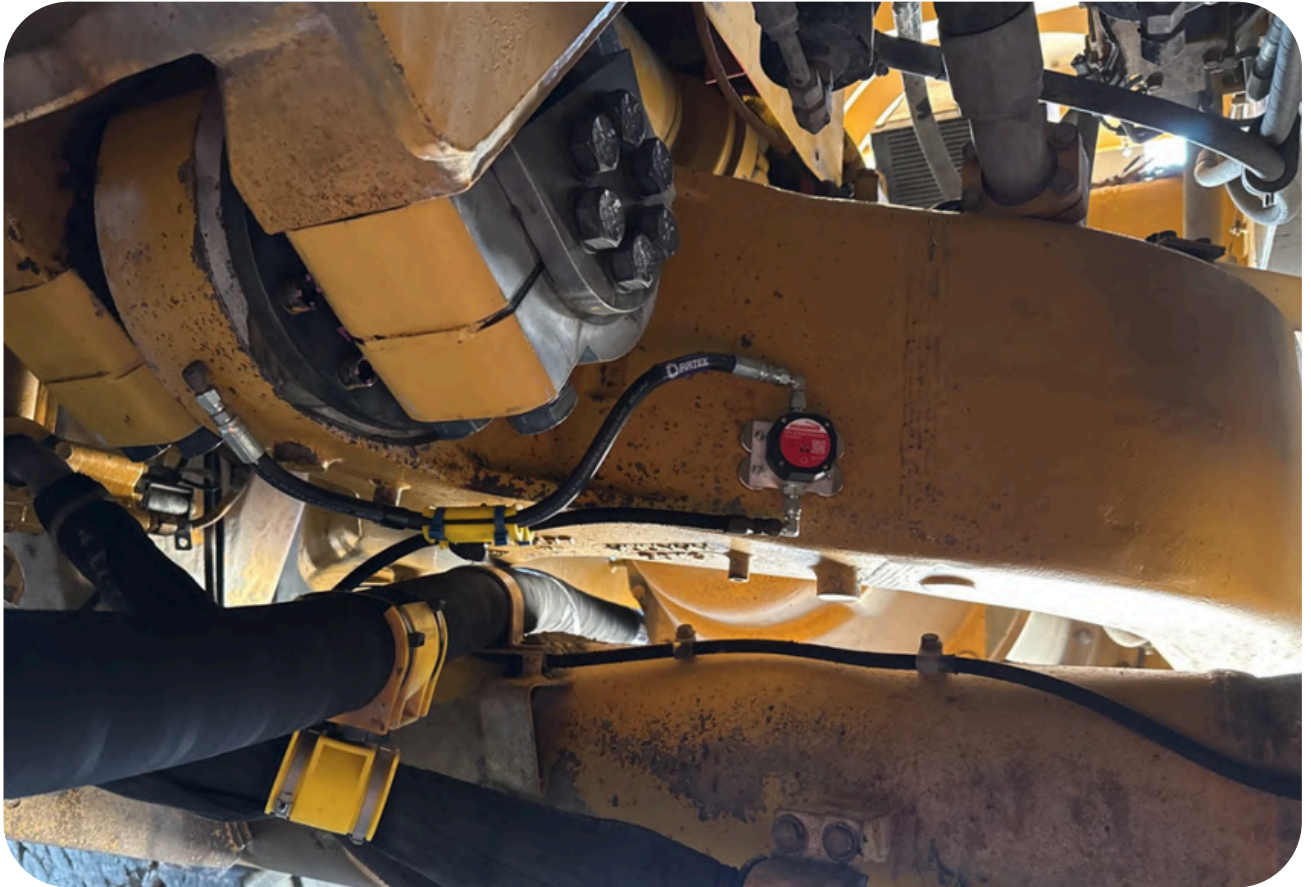
Endpoint Low Flow monitoring the A-frame bearing
