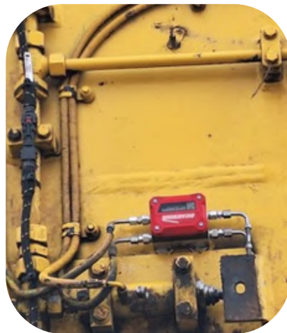
Endpoint MP2 monitoring bucket pins (LHS & RHS) – mounted on silicon magnets on the stick
