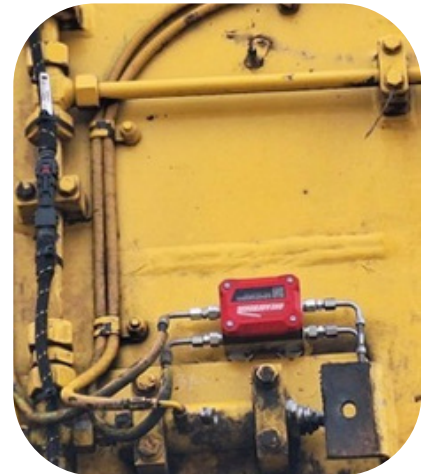
Endpoint MP2 monitoring bucket pins (LHS & RHS) – mounted on silicon magnets on the stick
