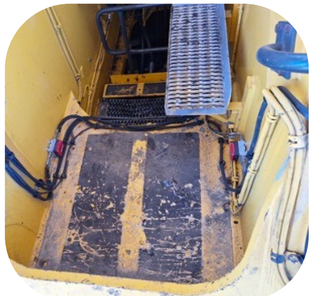
Endpoint MP2 monitoring hoist cylinders – mounted on silicon magnets in the "snake pit"
